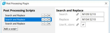
As this also removes your inital heating up of the nozzle, one should update the start script to include a ";INIT=WAIT FOR S{material\_print\_temperature\_layer\_0}"
