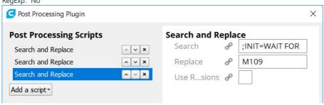
I didn't want to remove the original M109 S{material\_print\_temperature\_layer\_0} as this could have unwanted side-effects as I got pointed out lately that Cura does check if the start script contains the necessary temp preparation commands - else inserts them him/her-self after your own start script.
