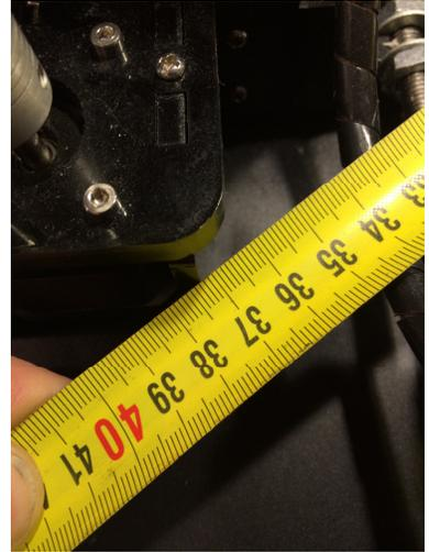
4. Crossmeasure from left back frame corner to right front motor mount, compare the number with measurement in point 3.
