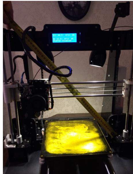
7. To make shure that x-axis guide bars are leveled to the frame (do not use water level)
