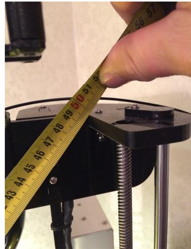
6. Crossmeasure from right motor mount to left top frame corner, compare the number with measurement in point 5.
