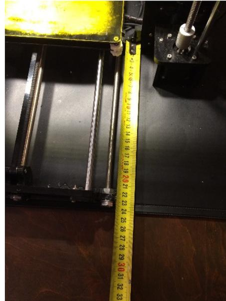
2. Measure left and right back to midsection, if the numbers are different loosen the nuts and make them exactly the same.
