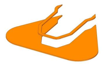
Using the assembled top & bottom plates of the printer as a template, mark where curves begin one at a time. Take a heat gun and using a back and forth motion, heat where the bend should be which will start to soften the plastic enough to shape it.
