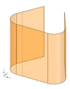
Glue the top and bottom flange to the cover using clear Plexiglas/acrylic glue
